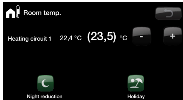
The example above shows that the room temperature is 22.4°C, but the desired value (setpoint) is 23.5°C.
